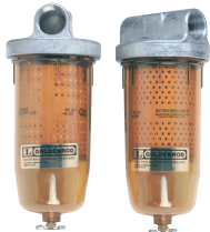
GOLDENROD WATER BLOCK FUEL FILTER, 9-1/2 X 4-IN. Removes water from fuels. 15 micron filtration, 5-gpm gravity flow with 24" head. (535 252)
